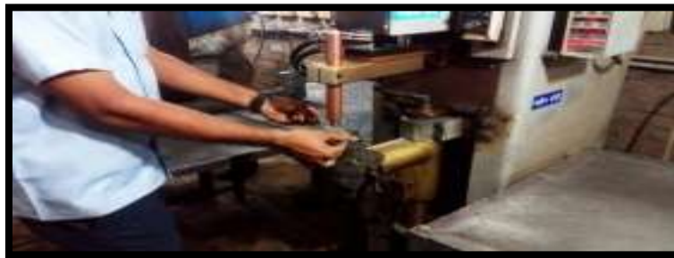
Figure 3.1: Resistance Spot welding Machine set up
